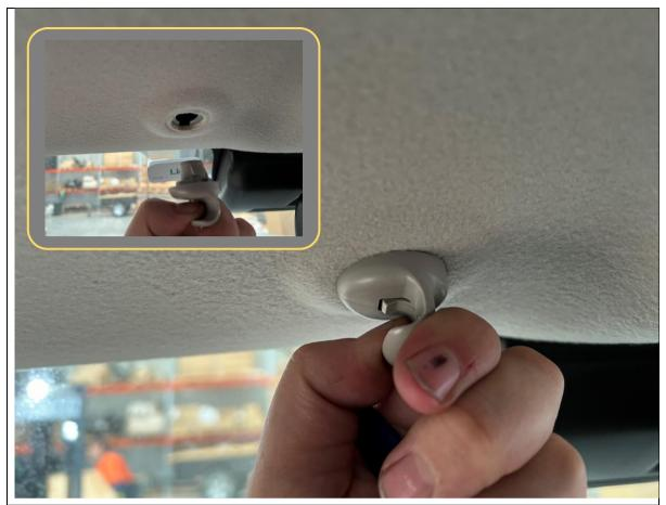
5. Remove sun visor keepers by rotating keepers 90 degrees and withdrawing from roof.
