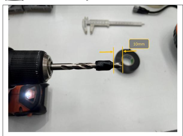
46. Insert 9mm drill into electric drill
